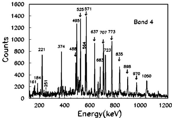
FIG. 3. Sum of clean double gates for the positive parity band of  $^{143}\text{Dy}$  (band 4). The in-band transitions are indicated with arrows. The linking transitions, as well as the low lying transitions fed by the band can also be seen.
