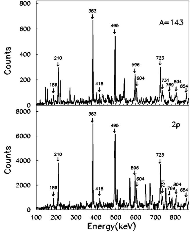
FIG. 1. Gamma-ray spectrum (not efficiency corrected) in coincidence with the 530 keV line ( $^{143}\text{Dy}$ ). (a) Gated with mass 143; (b) gated with particle fold  $2p$ . The peaks present in both spectra can be assigned to  $^{143}\text{Dy}$ . Their energy is shown in keV. The other peaks are contaminants from  $^{143}\text{Tb}$  in spectrum (a) and  $^{144}\text{Dy}$  in spectrum (b).
